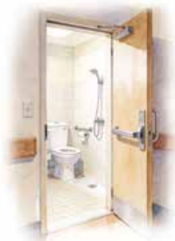
Bathrooms Opening Outside
